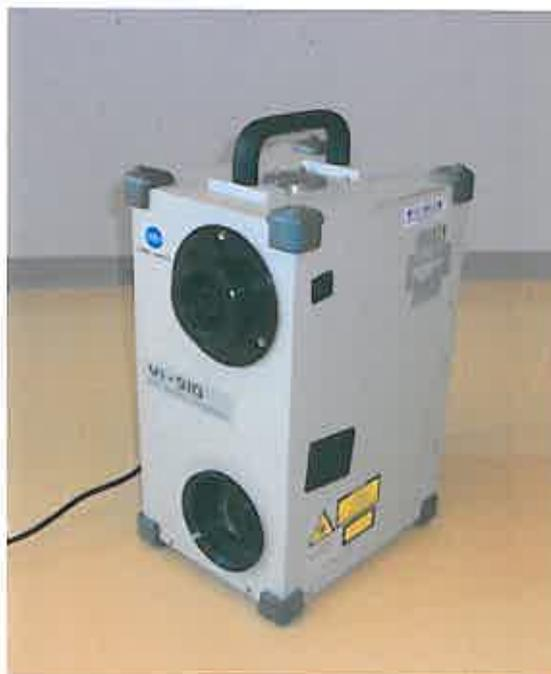
**Figure 13 : scanner laser**
